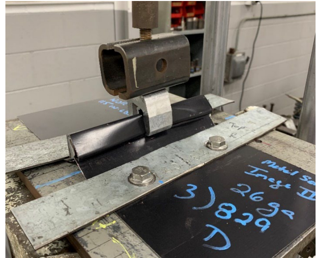
Figure 5: Standing Seam Clip Pull Test
