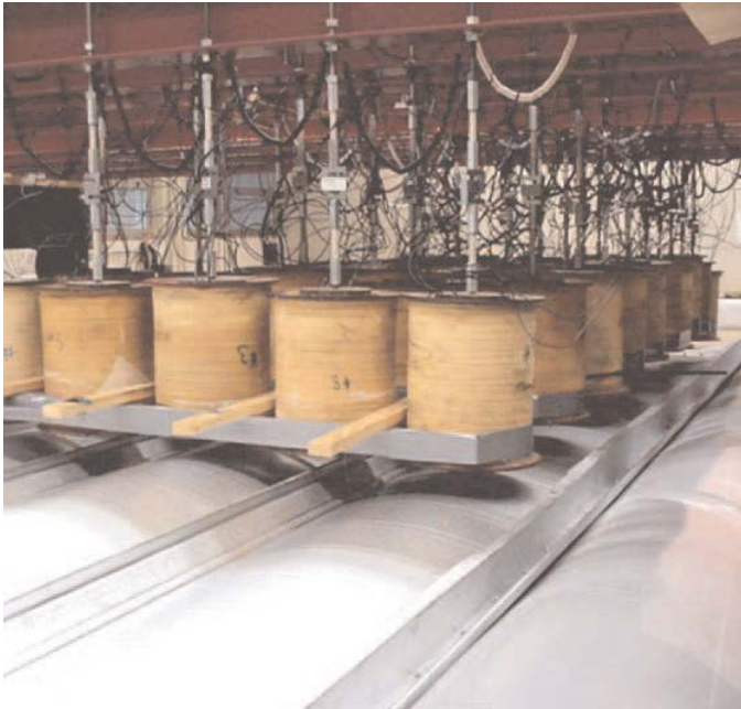
▲ Research funded by the Metal Building Manufacturers Association and American Iron and Steel Institute at Mississippi State University utilized electromagnetic fields to more accurately replicate the effects of wind on a roof surface. Photo courtesy of the Metal Building Manufacturers Association.
