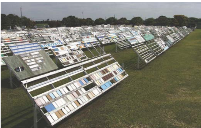
▲ Real-world exposure testing is the only infallible way to prove paint performance over time. South Florida is the favored test geography because of high heat, ultraviolet and moisture conditions. Photo courtesy of Atlas Weathering Services Group, Miami, FL.
